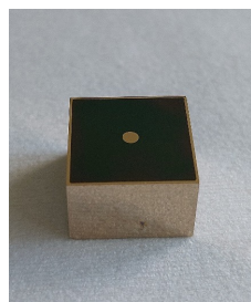
Hemispherical sensors with different volumes ( 10 \times 10 \times 5 \text{ mm}^3 , 15 \times 15 \times 10 \text{ mm}^3 , 20 \times 20 \times 10 \text{ mm}^3 ).
